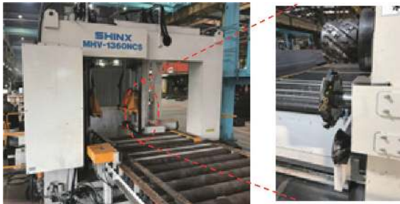
Photo 2 Five-sided processing machine for H-shapes
